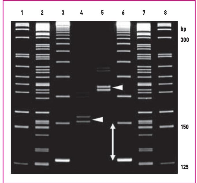
A vertical 8 cm long 8 % Acrylamide-Bis (29 : 1) gel containing 1X SeparateIT Polymer Solution was run at 200 V at identical conditions. Samples are identical to those loaded to the gel on the left. In the 25 bp ladder, the spacing between the 125 bp and 150 bp fragments increased 2.8 fold. The 151/155 and 183/187 bp alleles are fully resolved.
