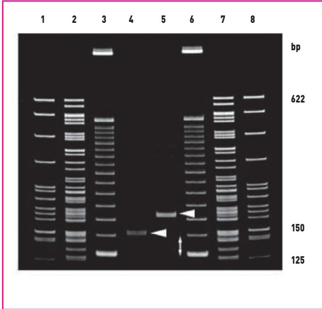
A vertical 8 cm long 8 % Acrylamide-Bis (29 : 1) gel was run at 200 V for 70 min. Lanes: 1,8 – pBR322/Msp I; 2,7 – M3 Marker; 3,6 – 25 bp ladder; 4 – vWA alleles 16 and 17 (151 and 155 bp); 5 – TH01 alleles 6 and 7 (183 and 187 bp). These microsatellite bands are not resolved.
