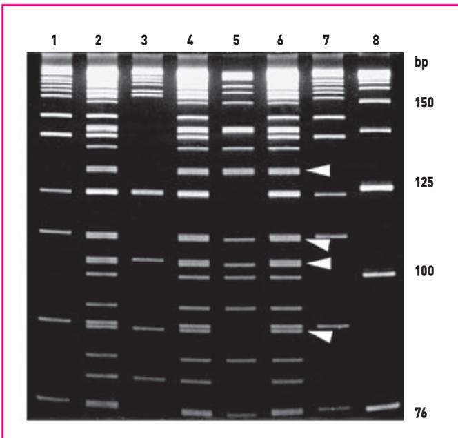
A vertical 8 cm long 11 % Acrylamide-Bis (29 : 1) gel containing 1X SeparateIT Polymer Solution was run at 200 V for 90 min. Lanes: 1,7 – pBR322/Msp I; 2, 4, 6 – M3 Marker; 3 – pBR322/Hae III, 7 – pBR322/Hha I, 8 – 25 bp ladder. The marked band pairs include 89/90, 103/104, 109/110 and 131/132 bp.
